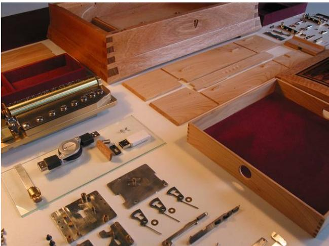
Work started with a mixture of pencil-on-paper sketches, written ideas and discussions. With the expansion of the project into a set of 7, it was decided that every aspect of the work would be custom made, included all the metalwork - from the hinges to the locking systems. The designs were then extensively developed into a series of detailed drawings using computer aided drafting (CAD).
