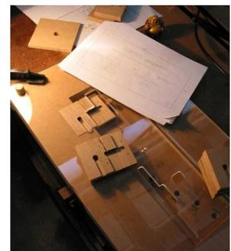
Inside the boxes, the complex locking mechanisms are embedded within precise cavities and hollows cut into the walls. Since it was not possible to put the wall sections directly onto the CNC router to cut these cavities, we instead had the CNC routing machine make us a special set of guides and templates, allowing us to cut the precise cavities in the workshop using a manual routing set-up.
