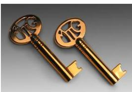
Two keys were made for this box. The head of each key is laser-pierced with the initials 'MTG'. The parts of the keys were silver-soldered together and the 'bit' of each key was filed by hand to precisely mate with the lock's tumblers.
